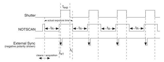
Figure 18. Frame Transfer where Pulse arrives after Readout
